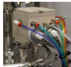
The modules are constructed of materials suitable for autoclave sterilization and, after taking a sample, the module is sanitized using a liquid sanitant.
